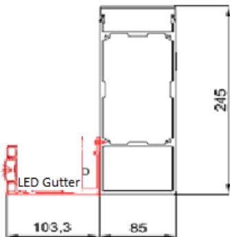
Fig. 1A. Lighting kit in pergola SB400PRO - location marked in red. (1 -LED gutter with LED strip; 2- LED bar (when 2 gutters) or LED gutter (when 4 gutters); 3- LED gutter plugs; 4- lighting controller (White LED Receiver); 5- 24VDC power supply, 6- pen with light points; 7- cable to bar+at opposite ends: plug and power cable)
